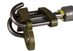
Wire Grip Grips conductor, has hole for block or line hook. WWL for grips 1,000 lb (454 kg) at a 4:1 ratio. 3600Q-ES • Opening min. 0.3125 in max. 0.875 in 2 lb • (7.9 mm, 2.2 cm) • (0.91 kg) 3601Q-ES • Opening min. 0.5 in max. 1.5 in 3 lb. • (1.3 cm, 3.8 cm) • (1.36 kg)
