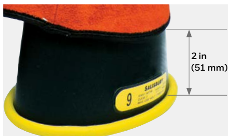
Minimum distance from the leather protector cuff to the bead of the rubber glove for this Class 2 glove is 2 in (51 mm).
