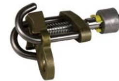
Wire Grip Grips conductor, has hole for block or line hook. WWL for grips 1,000 lb (454 kg) at a 4:1 ratio. 3600Q-ES • Opening min. 0.3125 in max. 0.875 in 2 lb • (7.9 mm, 2.2 cm) • (0.91 kg) 3601Q-ES • Opening min. 0.5 in max. 1.5 in 3 lb. • (1.3 cm, 3.8 cm) • (1.36 kg)
