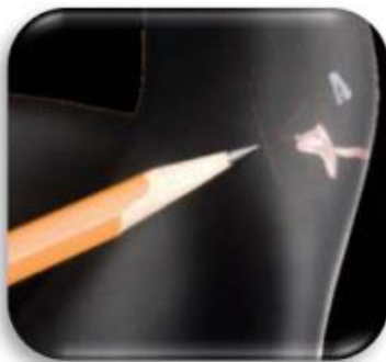
Splits, cuts or holes from snags and punctures
