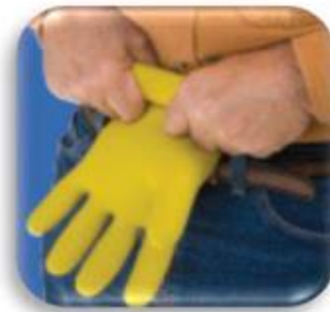
7. Turn glove inside out and repeat the process
