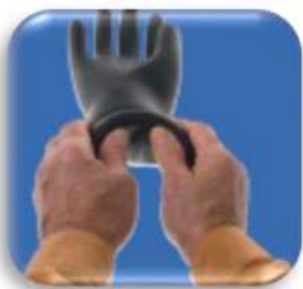
4. Twirl glove, rotating on rolled ends
