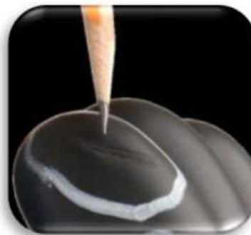
Grooves worn due to rope burns or heat exposure
